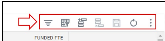
Figure 9 Every sheet has a toolbar with Filter, Display Options, Add/Remove rows, Save (diskette), and other options.
